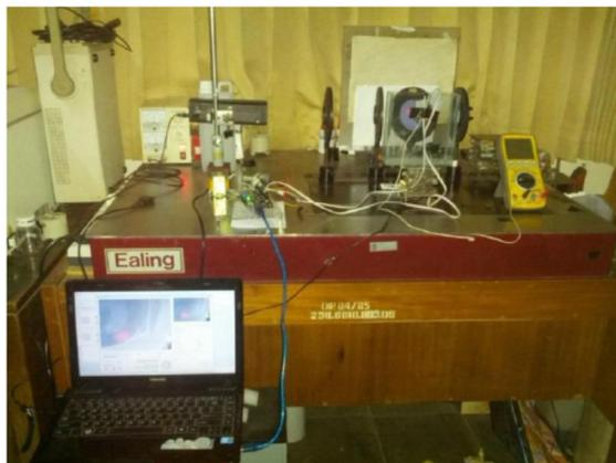
**Gambar 3.9 Sistem Interferometer Michelson *Real Time*.**
