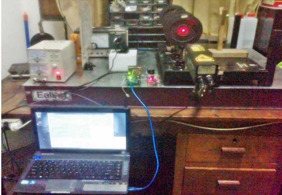
Gambar 8. Keseluruhan Set Up Alat Interferometer Michelson *Realtime*
