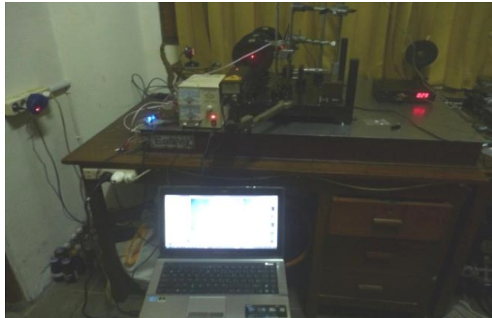
Gambar 9. Set Up interferometer Michelson real time
